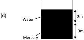
If the density of mercury is 13600kgm<sup>-3</sup> and the density of water being 1000kgm<sup>-3</sup>. Calculate the pressure exerted at point A.
