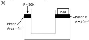
Calculate the weight of the load.
