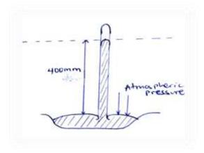
Calculate the atmospheric pressure
