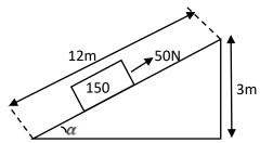
A load of 150N is raised on an inclined plane through a distance of 3m by an effort of 50N that moves through a distance of 12m. Calculate
